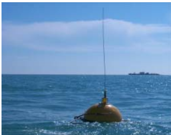
Site-specific measurements to ensure that wave criteria used for engineering purposes are fully validated
